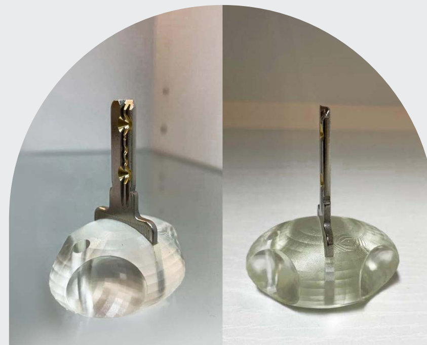
A 3D printed key holder designed to ease key pick up for clients with restricted fingers mobility.
